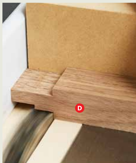
Raise the blade to \frac{3}{8} " above the table and rabbet the top face of each side rail (D).
