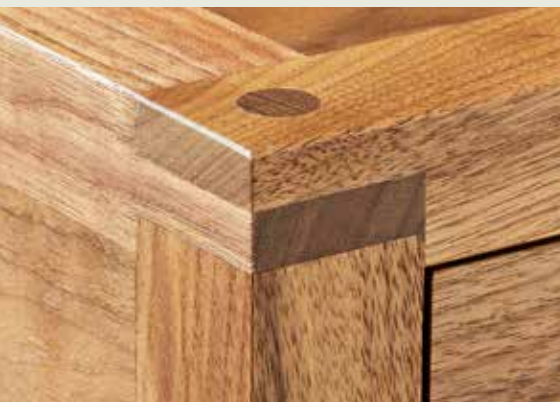
With the pieces on a flat surface, the top faces should be flush, with the mating faces of the lap touching and the ends and edges flush.
