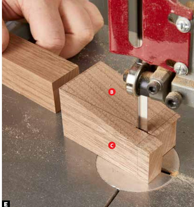
E Mark the taper on the just-sawn face and bandsaw it. Sand both tapers smooth.
