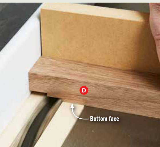
Attach an auxiliary fence to your miter gauge to prevent chip-out. Set the blade \frac{1}{4} " above the table, and rabbet the bottom face of each side rail (D).
