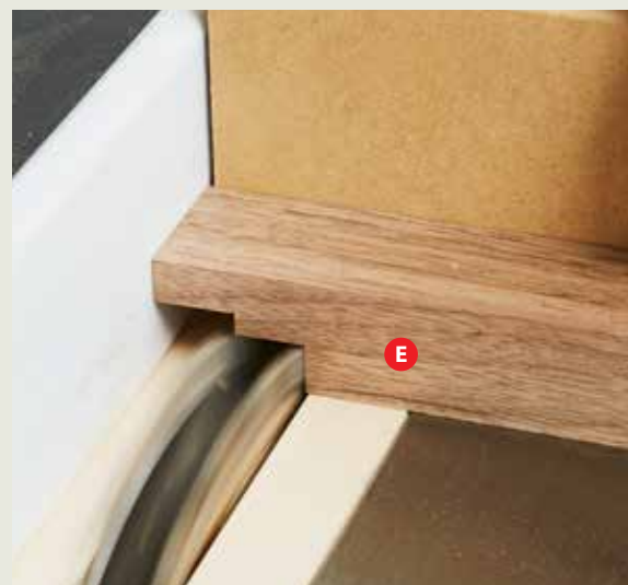
Raise the blade to \frac{3}{8} " and rabbet the bottom face of the front and back rails (E).
