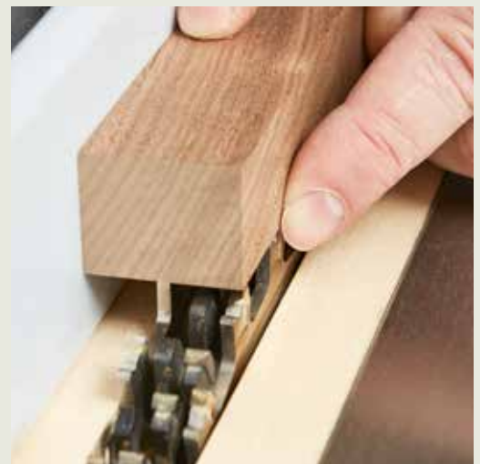
Use one of the test pieces to set your rip fence so the outside edge of the piece is flush with the outside tooth of the blade.
